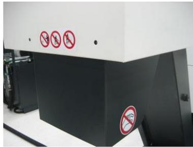
G.2 Parts operated by opening or releasing the interlock of a guard
