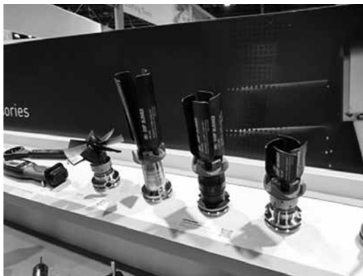
(b) Big社のAutomatic cleaning Chip Blower
